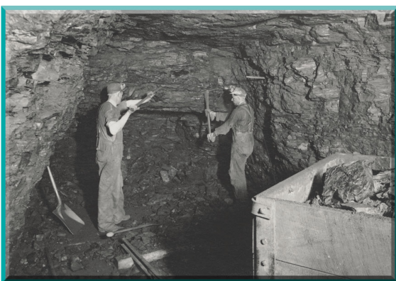
Figure 7. Miners digging coal with a pick ax and shovel in a WLCC mine near Wilton, North Dakota. (SHSND 0410-181a)
