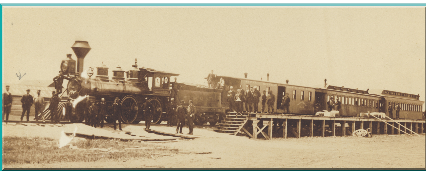
Figure 2. A train, consisting of a 4-4-0 locomotive, a baggage car, and two passenger cars, belonging to the St. Paul, Minneapolis, and Manitoba Railway, stopped at the passenger platform at the station in Arvilla, North Dakota, ca. 1882. This railway later became the Great Northern. (SHSND B0060)
