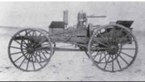
Tiller Stick Automobile. This car was made by Frank Jaskowiak of Bismarck in 1902. It has a tiller stick for steering. (SHSND A5595)
